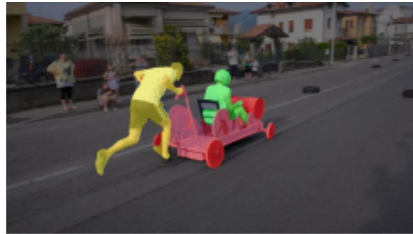
Figure 4. An example of DMM-Net's video object segmentation: The runner, cart, and rider are all determined "objects" while the background is not.
