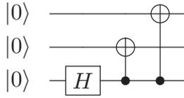
FIG. 2. Circuit used to generate the three-qubit GHZ state on IBM’s superconducting quantum computation platform.
