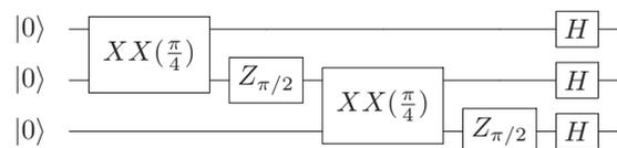
FIG. 1. Circuit used to generate the three-qubit GHZ state in the trapped ion system. The  $XX$ -gate action is given in Eq. (17).
